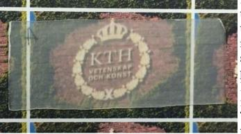
through the wood more directly, the researchers incorporated acrylic, often known as Plexiglass. The researchers could see through the resulting material, which was twice as strong as Plexiglass. Although the wood isn't as crystal clear as glass, its haziness provides a possible advantage for solar cells. Specifically, because the material still traps some light, it could be used to boost the efficiency of these cells, the scientists note.
