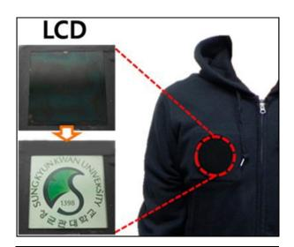
A new kind of material can harness energy from human movement and use it to light up a small LCD display. Credit: American Chemical Society
